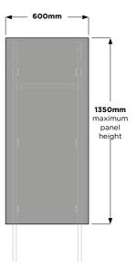
Impact frames with pre-fitted universal fixing clips are based on these standard panel divisions, however clips can be relocated to suit alternative dimensions. Alternatively Impact Core Range Units can be purchased without pre-fitted universal fixing panel clips if required.
