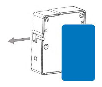
The Locker is not occupied and the shoot bolt is inside the lock.
