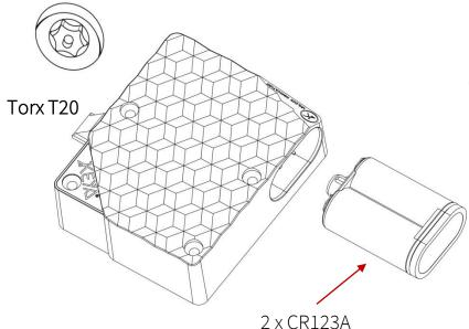
To release the battery holder turn the T20 screw.
