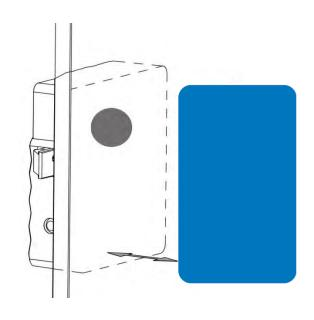
The shoot bolt will extend out, moving to the locked position.
