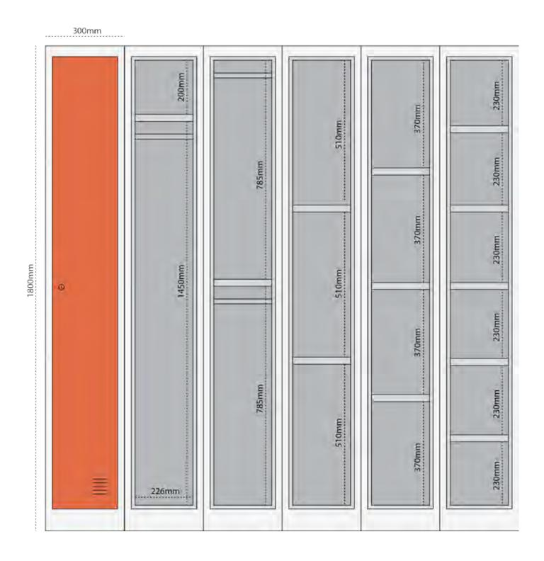
Interior dimensions shown above detail the size of the door opening, the actual internal space will be larger.
